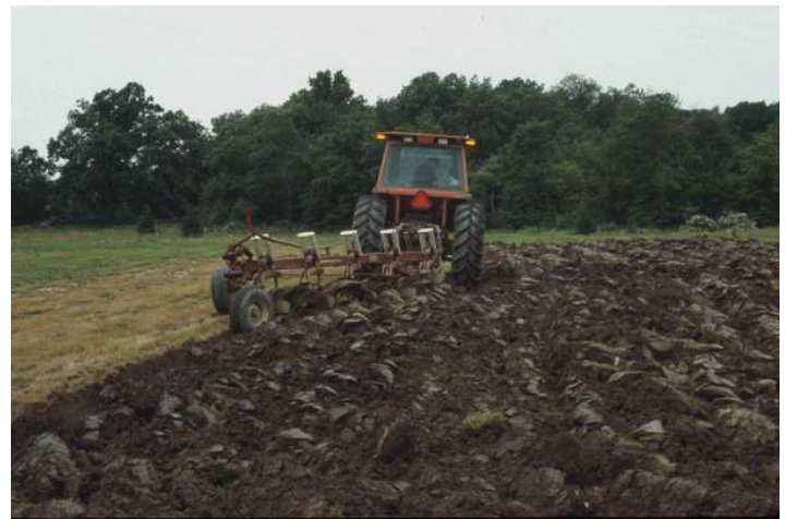
Fig. 2 Tumbling of the soil behind a moldboard plow forces with soil clay's multi-layered structure and bonding forms. With long periods of rest when not being tilled, the soil matrix will have an opportunity to reform into specific structural units. Tillage events will continue to break down soil structure into a condition of disarray where the soil melts together into something akin to concrete-like soil structure due to excess tillage.
